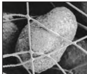
Gas contaminants must pass through tortuous pathways coming in intimate contact with the carbon.
