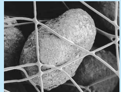
Gas contaminants must pass through tortuous pathways coming in intimate contact with the carbon. The fibers anchor themselves to the carbon using only 1% of the carbon's surface helping to maximize the contaminant's exposure.
